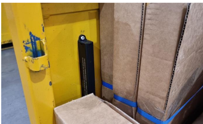
Parcel Cage with IoT Tracking Device connected to Thinxtra's 0G Network
